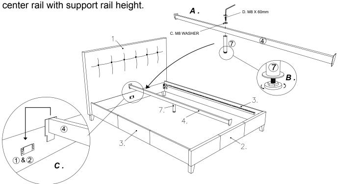
**Please Note**: Do not tighten any bolts until all components (Part 1, 2, 3 & 4) are in place.
